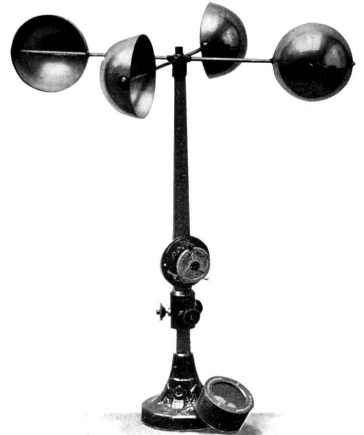
THE ROBINSON ANEMOMETER.
